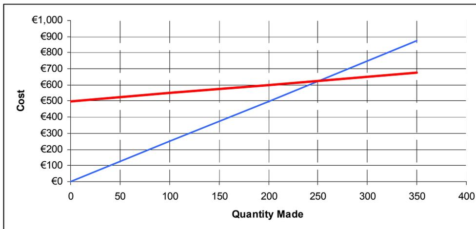
From the graph, determine the set-up cost for automation and the quantity of face guards required to justify the decision to automate (Break Even Quantity).
