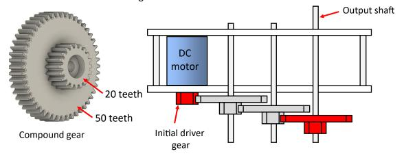
If the motor runs at 2000 rpm, calculate the angular velocity (rotational speed) at the output shaft.
