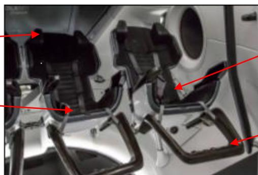
Seats are measured to fit the operator; they can tilt back into a flat configuration.
