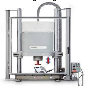
Accelerated can be carried out on the buttons of a computer mouse by automatically simulating repetitive actions of pressing the buttons on a fatigue testing machine.
