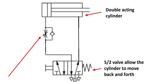
(ii) Flow control valve, slow speed of the ram moving forward, with unrestricted speed on return.
