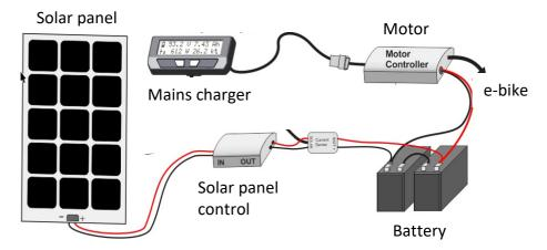
Solar charging will require solar panel to capture solar energy, controller and sensor systems to process the electrical charge. The battery will collect, store and distribute energy for the e-bike.
