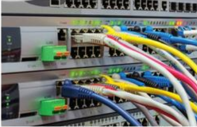
▲ Figure 5.7 Cat5e cable is used to connect devices through their NICs
