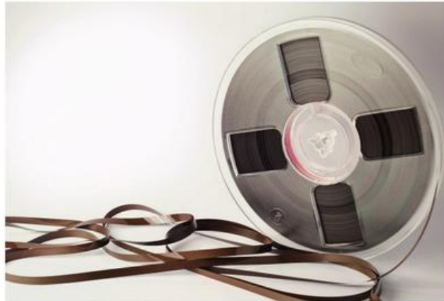
▲ Figure 1.76 Magnetic tape is mainly used for backing up data in large organisations
