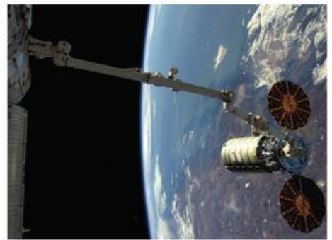
▲ Figure 2.16 Astronauts on the International Space Station use control software to move a robotic arm into position in order to capture a supply capsule
