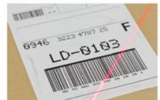
► Figure 1.44 Linear barcode used to identify a parcel
