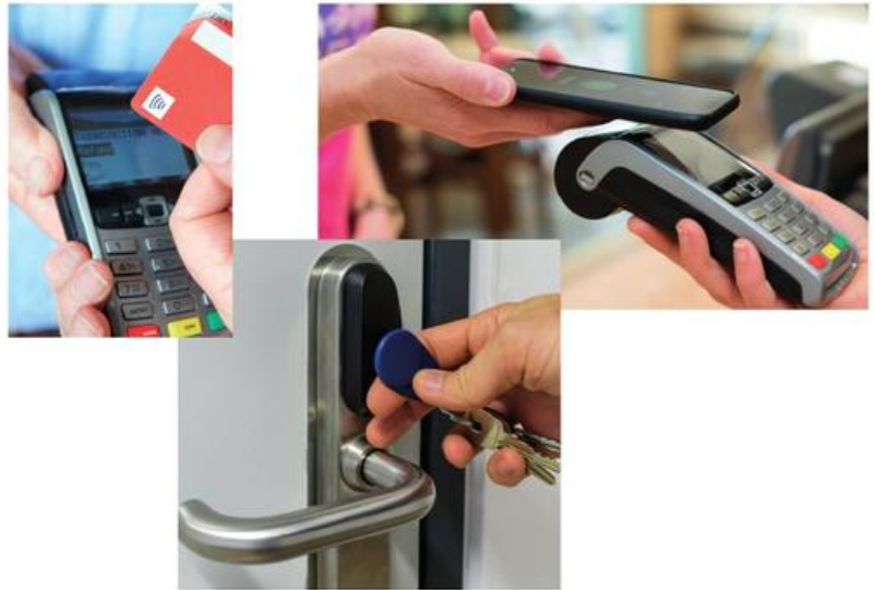
▲ Figure 1.58 RFID tags can be included in a variety of objects
