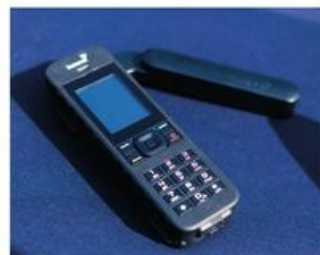
▲ Figure 4.11 Satellite telephones use antennae to transmit data to (and receive data from) one or more satellites
