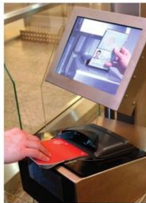
▲ Figure 1.55 Some passports now contain a chip that holds biometric data about the passport holder that is compared with the results of biometric scans carried out at airports
