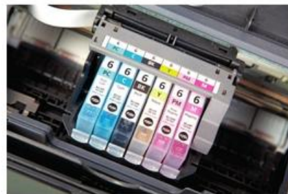
▲ Figure 1.64 Cartridges used in an inkjet printer
