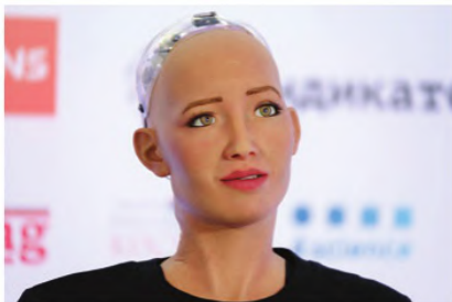
▲ Sophia, a humanoid robot. She uses voice recognition (speech-to-text) technology and is designed to learn over time. Her AI program analyses conversations and extracts data that allows it to improve responses in the future
