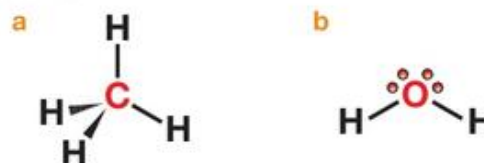
▲ Figure 8.12 (a) A methane molecule is tetrahedral and (b) a water molecule is bent.
