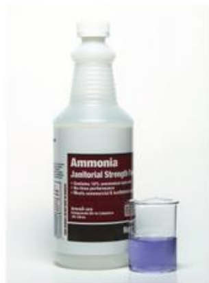
▲ Figure 16.5 Ammonia solution is sometimes called ammonium hydroxide. It is an alkali and is used in some cleaning products. Some universal indicator solution has been added to it in the beaker.
