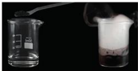
► Figure 20.20 The beakers both contain hydrogen peroxide solution, the right-hand one has \text{MnO}_2 added to speed up oxygen production.
