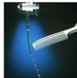
▲ Figure 8.13 Water being bent by an electrically charged comb.
