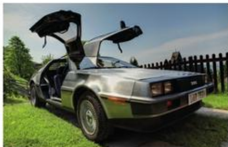
▲ Figure 15.13 Some cars have a stainless steel body. They do not need to be painted.
