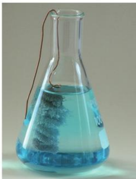
▲ Figure 14.7 Displacing silver from silver nitrate solution
