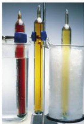
▲ Figure 21.8 Tubes containing the \text{NO}_2/\text{N}_2\text{O}_4 equilibrium at different temperatures.
