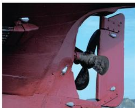
▲ Figure 14.19 A sacrificial anode on a ship
