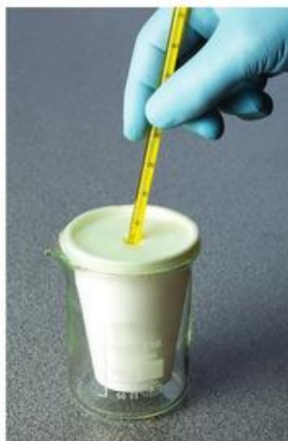
▲ 19.12 A calorimetry experiment to measure the enthalpy change of a displacement reaction.
