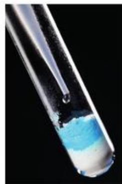
▲ Figure 18.3 Testing for water with anhydrous copper(II) sulfate.
