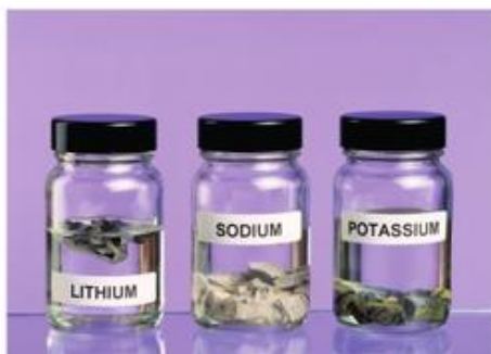
▲ Figure 11.4 Lithium, sodium and potassium have to be kept in oil to stop them reacting with oxygen in the air.
