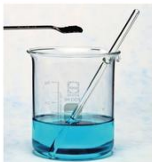
▲ Figure 16.6 Copper(II) oxide reacts with hot dilute sulfuric acid to form blue copper(II) sulfate solution.
