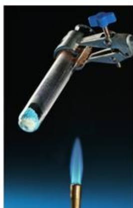
▲ Figure 21.1 Copper(II) sulfate crystals are split into anhydrous copper(II) sulfate and water on gentle heating.
