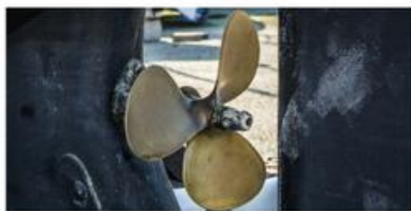
▲ Figure 15.6 A brass propeller. Brass is an alloy.
