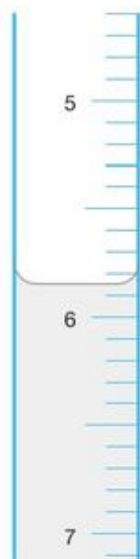
▲ Figure A2 Measuring from the bottom of the meniscus.
