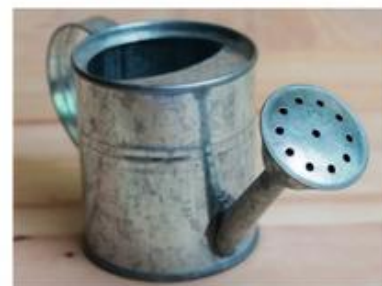
▲ Figure 14.18 Galvanised iron doesn't rust even in constant contact with air and water.
