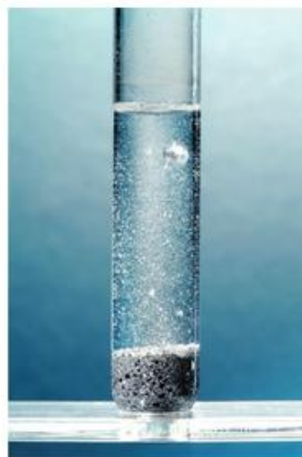
▲ Figure 14.15 Iron reacting with dilute hydrochloric acid
