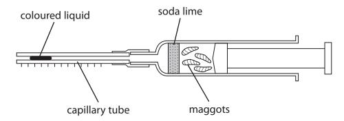
This respirometer can be used to investigate the uptake of oxygen during the respiration of maggots.
