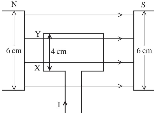
Which of the following is the force on side XY if the current in the wire is 2.0 A?
