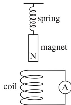
The magnet is pulled down until its north pole is just at the top end of the coil. The magnet is released and initially accelerates upwards away from the coil.
