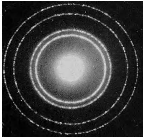
In a particular investigation the atomic spacing of the crystal is  $2.3 \times 10^{-11}$  m and the electrons are accelerated through 3000 V.
