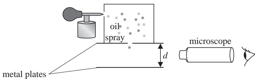
Negatively charged oil drops are sprayed into a region above two parallel metal plates. The plates are separated by a distance  $d$ . The oil drops are allowed to enter the region between the two plates.
