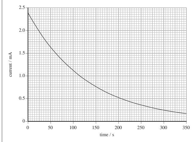
(i) Show that the capacitance of the capacitor is about 0.02 F.
