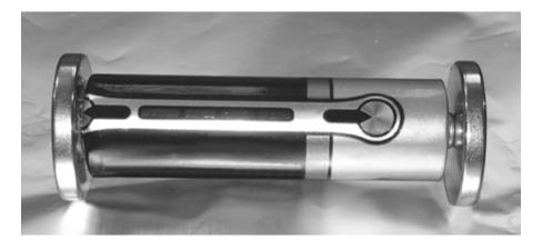
When the motor is placed on an aluminium sheet, the motor begins to roll.
