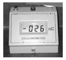
The charge the coulombmeter is measuring is stored on a capacitor inside the meter. A voltmeter inside the coulombmeter measures the potential difference across the capacitor. This value is converted so that the display shows the charge in nanocoulomb.
