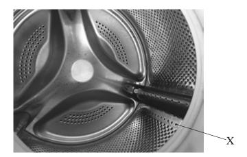
The drum is a hollow metal cylinder with a series of holes through its surface. During the spin cycle the drum rotates at 1400 revolutions per minute to separate the water from the wet clothes.
