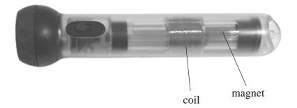
Inside the torch is a coil of wire and a magnet that can move freely through the coil in alternate directions when the torch is shaken. The coil is connected to a rechargeable battery.
