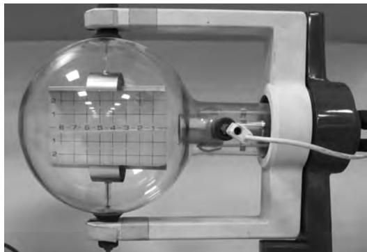
In the tube the path of a beam of electrons can be observed on a grid. The grid is positioned between two metal plates with a potential difference (p.d.) across them.
