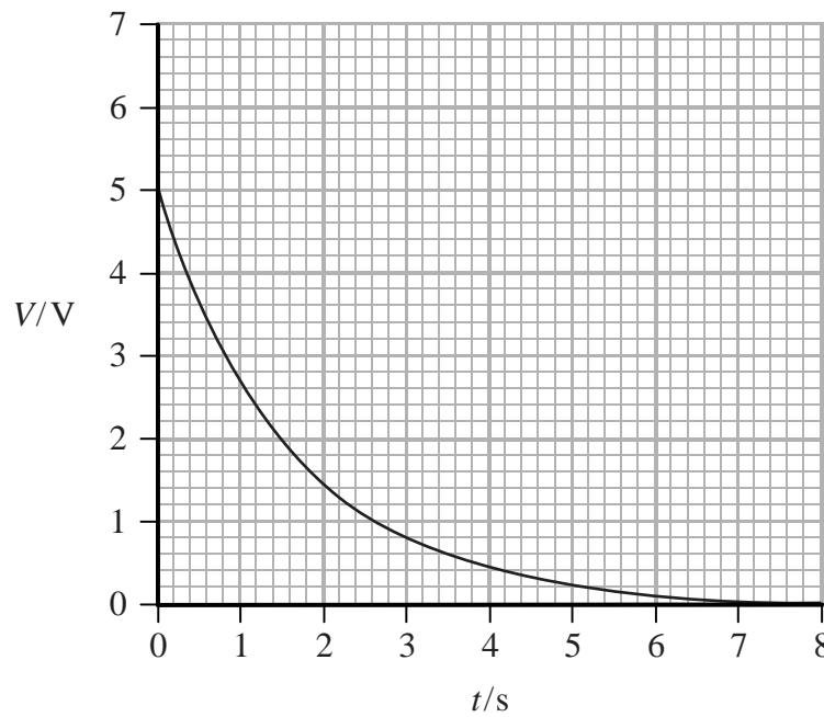
Show that the capacitance of the capacitor is about  $2\text{ mF}$ .
