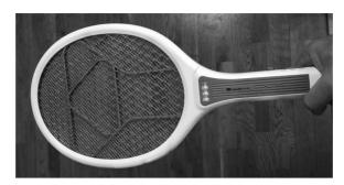
The racquet has two metal meshes. When a fly is between the meshes, the user presses a button and a potential difference (p.d.) of  $1500\,\mathrm{V}$  is applied between the meshes for a short time. This p.d. causes a current in the fly, stunning it.
