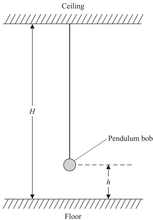
The student measures the distance  $h$  from the floor to the centre of the pendulum bob. He determines values of the time period  $T$  of the pendulum for different values of  $h$ .
