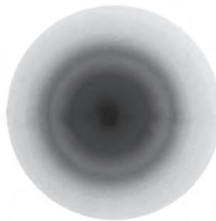
By measuring the diameter of the rings it is possible to calculate a value for the wavelength  $\lambda$  of the electrons from
