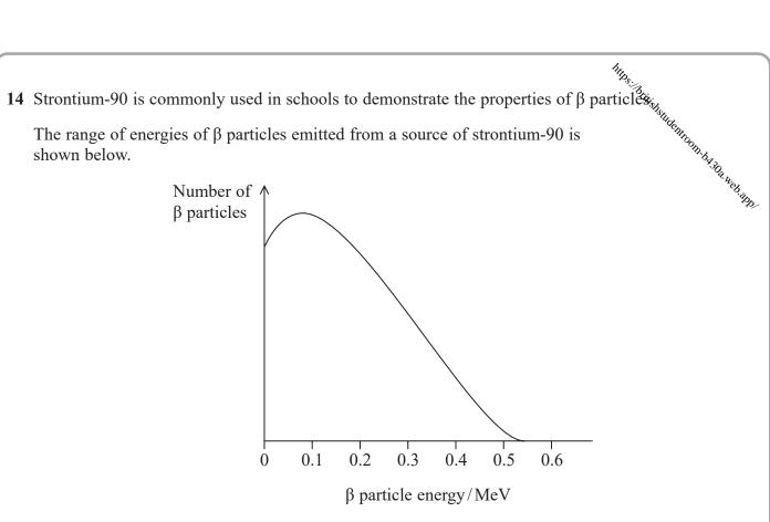
When  $\beta$  particles travel through air they ionise air molecules, which limits how far they travel. The range of the β particles depends upon their kinetic energy when released from the nucleus.
